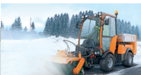
B series with front sweeping brush and roller combi spreader
