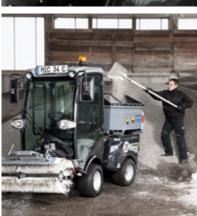
Parallelogram-led sweeping system The freely suspended sweeping mechanism with unloader and hydraulic floating posi-
