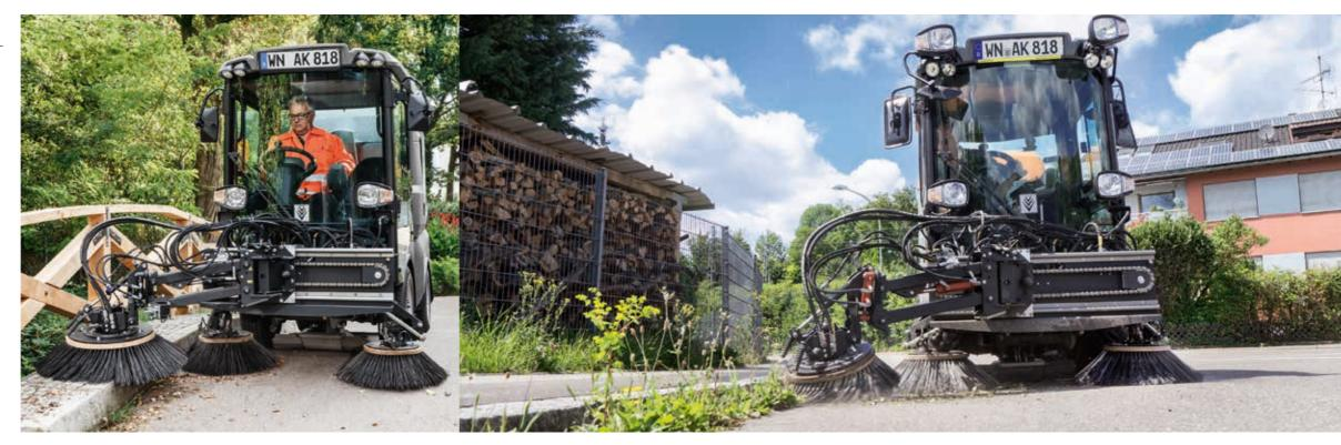
A weed brush installed on the third brush arm can remove weeds effectively, thanks to the running rail across the entire machine width, for example on footpaths or cycle paths or in access areas to residential areas or parks. The three-brush system therefore offers you a number of applications at no extra cost.
