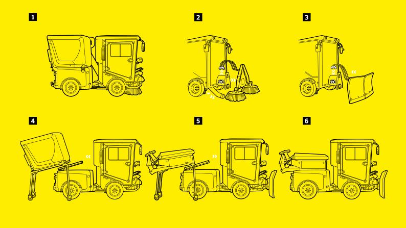
Our integrated quick-change system for front and rear implements allows one person to effortlessly change implements and reduces the set-up times, thus making applications much more flexible.
