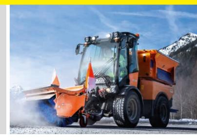
The Holder S 75 has all this and more. Its articulated steering provides the agility, precision and tracking required for perfect results. The permanent all-wheel drive optimally distributes the power of the 75 hp engine to all four wheels. The compact width of minimum 1.31 m (depending on tyres) enables you to reach every nook and cranny in town. And, best of all, from the comfort of your cab, you can steer through even the toughest jobs with ease.
